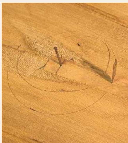
Phil's 'high-tech' solution for cutting clean, accurate circles!
